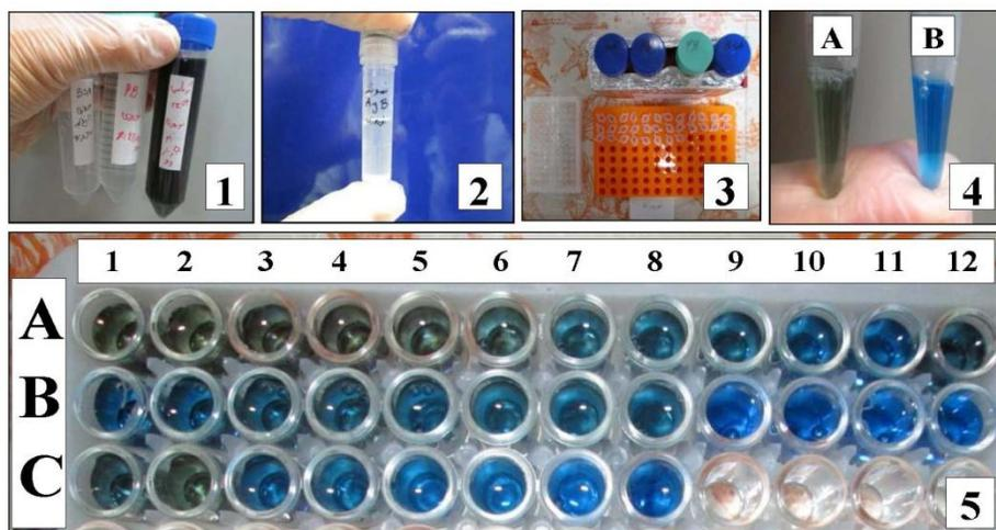
**Figure 2.** Materials and the reactions in Bradford microplate protein assay; Standard source, phosphate buffer and reagent (1), sample (Ag B) (2), preparation of blank, standards and sample dilutions in 0.5 ml tube (3), the reaction of assay reagent and BSA standard (assay reagent (A), the mixture of assay reagent with BSA standard (B))(4), the dye reaction of blank, BSA standards and sample dilutions (codes are according to Table 1 and Table 2) (5).
